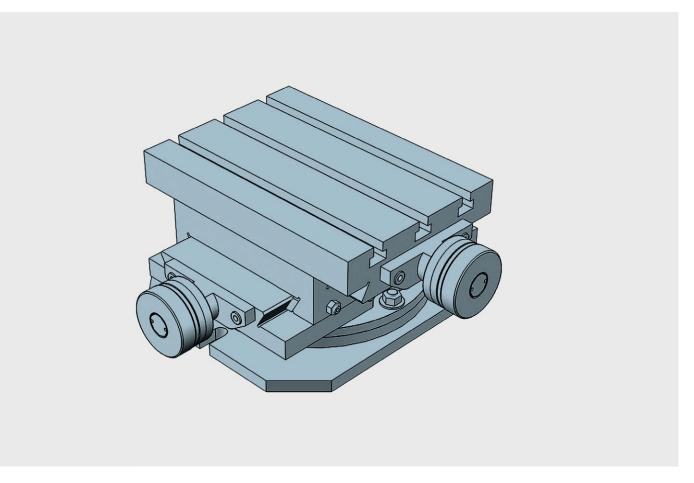
Double axis crosstable with rotary basis: the swivel support base comes with 180° in order to carry out angled works. All elements in stabilized cast iron GG25. All surfaces with grinded finishment. Millimetered rules in XY. Vernier/nonuis matt chrome. Dial, with zero setting. Spindle with triangular thread. Adjustable spindle nut. Standard lock in XY (M6 screw to block the dovetailed guides in working position)
