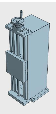
VERTICAL axis table for applications with linear units. Can be used only in vertical position All elements in stabilized cast iron GG25. All surfaces with grinded finishment. Millimetered rules in XY. Vernier/nonuis matt chrome. Dial, with zero setting. Spindle with trapezoidal thread. Adjustable spindle nut. Standard lock in XY (M6 screw to block the dovetailed guides in working position)
