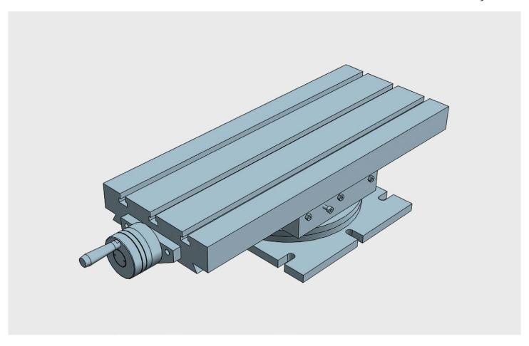
SINGLE axis table with rotary table (180°) for applications with linear units. Can be used in horizontal or vertical position All elements in stabilized cast iron GG25. All surfaces with grinded finishment. Millimetered rules in XY. Vernier/nonuis matt chrome. Dial, with zero setting. Spindle with trapezoidal thread. Adjustable spindle nut. Standard lock in XY (M6 screw to block the dovetailed guides in working position)
