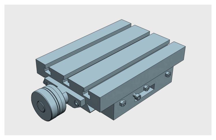
SINGLE axis table for applications with linear units. Can be used in horizontal or vertical position All elements in stabilized cast iron GG25. All surfaces with grinded finishment. Millimetered rules in XY. Vernier/nonuis matt chrome. Dial, with zero setting. Spindle with triangular thread. Adjustable spindle nut. Standard lock in XY (M6 screw to block the dovetailed guides in working position)
