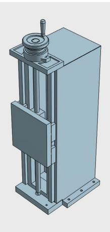
VERTICAL axis table for applications with linear units. Can be used only in vertical position All elements in stabilized cast iron GG25. All surfaces with grinded finishment. Millimetered rules in XY. Vernier/nonuis matt chrome. Dial, with zero setting. Spindle with trapezoidal thread. Adjustable spindle nut. Standard lock in XY (M6 screw to block the dovetailed guides in working position)
