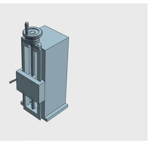
VERTICAL axis table for applications with linear units. Can be used only in vertical position All elements in stabilized cast iron GG25. All surfaces with grinded finishment. Millimetered rules in XY. Vernier/nonuis matt chrome. Dial, with zero setting. Spindle with trapezoidal thread. Adjustable spindle nut. Standard lock in XY (M6 screw to block the dovetailed guides in working position)
